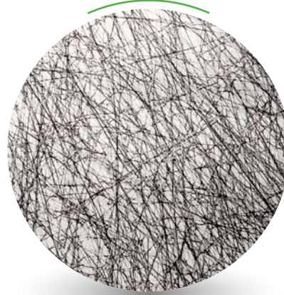
Bonding by calender and/or flow through oven by melt adhesive fiber (Bico or PP)
